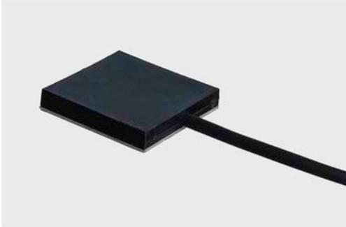
The surface temperature sensor (STS) is designed for temperature measurements on surfaces. Installed at the back of a solar module, the STS measures the module's temperature. The temperature of the solar modules is crucial for their output which decreases by 0,43 % per Kelvin with increasing temperature (typical value for mono- and polycrystalline modules).
